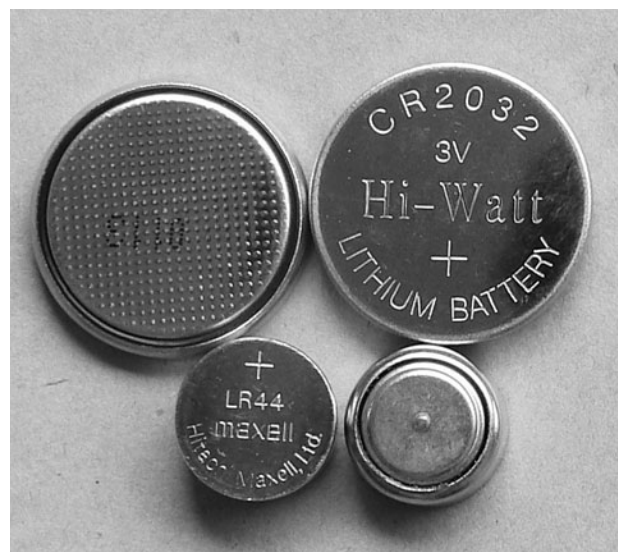
Figure 1-4 The smaller LR44 cell is an alkaline battery. The bigger CR2032 cell is a lithium battery.
