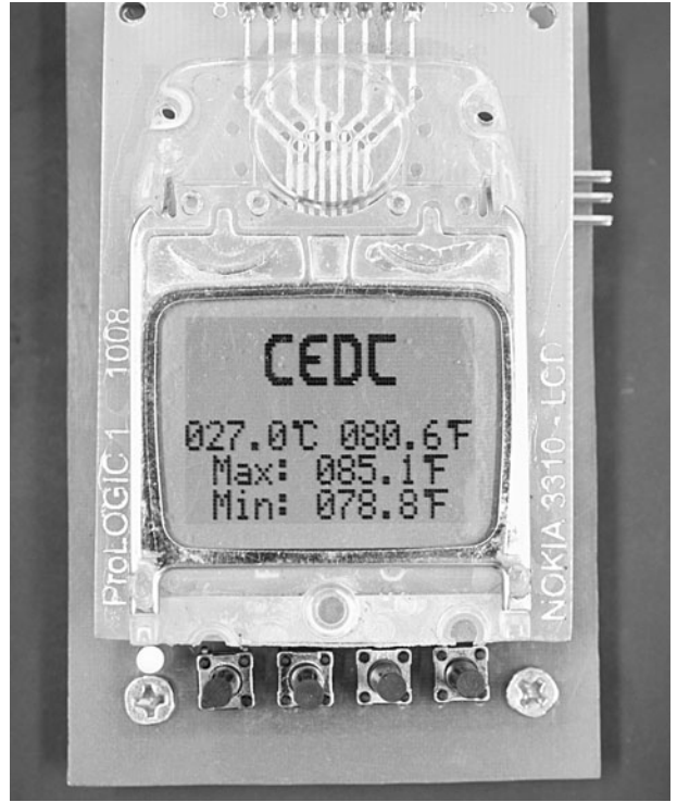
Figure 4-7 Temperature plotter display in readout mode
